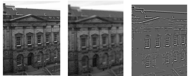
Figure 4: The original image is shown on the left, the low-frequency image in the middle, and the high frequency image (normalised) on the right.
